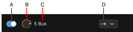
A. Bypass B. Send level C. Send destination D. Tap point (Input, Pre Fader, or Post Fader)
