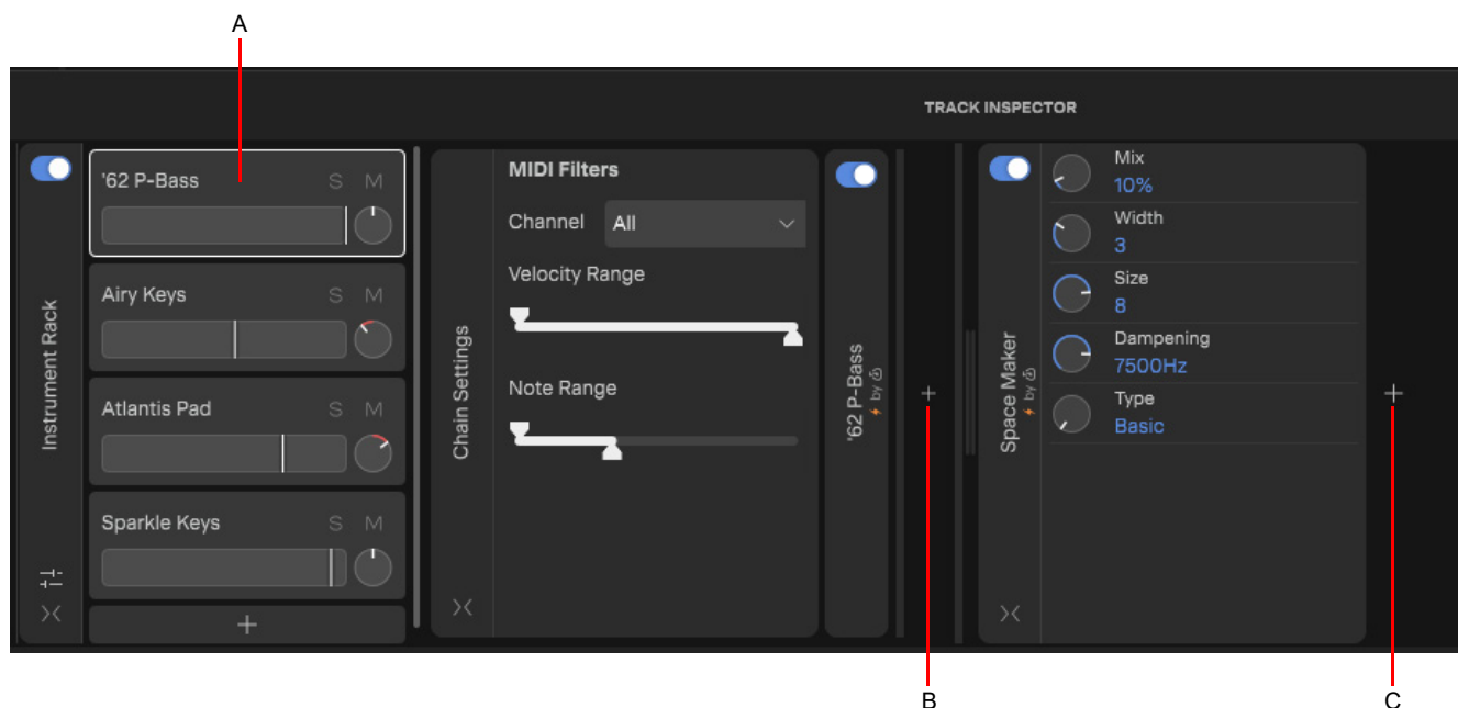
A. Selected instrument B. Add effects to selected instrument slot C. Add master effects to entire Instrument Rack
