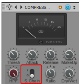
Figure 442. Add the PC4K S-Type Bus Compressor module in order to use sidechaining.
