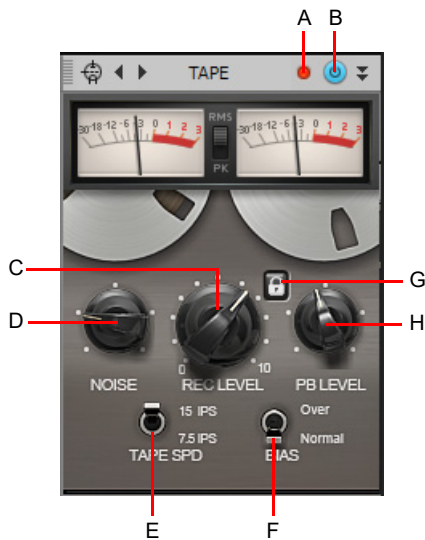
A. Clipping LED B. Tape Emulator enable/disable C. Rec level (input gain) D. Noise (tape hiss) E. Tape speed F. Bias G. Link H. Playback level
