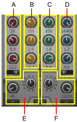
A. Low band (red) B. Low-Mid band (yellow) C. Mid-High band (green) D. High band (blue) E. High Pass filter (black) F. Low Pass filter (black)
