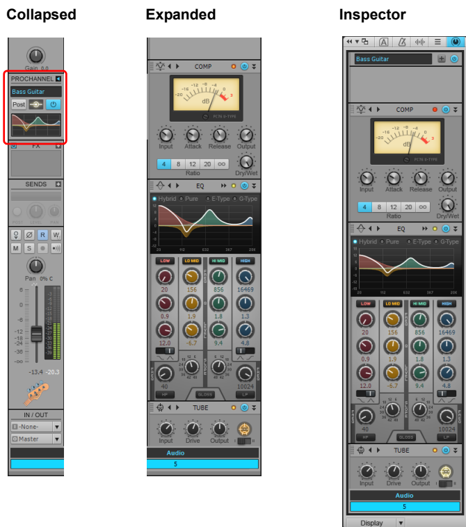
Figure 445. ProChannel can be displayed collapsed or expanded in the Inspector and Console view.
