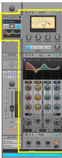
Figure 436. ProChannel provides compressor, equalizer, tube saturation, console emulation, tape emulation, and convolution reverb processing for each channel.
