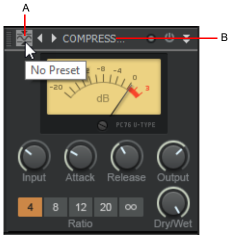
A. Category type icon (click to open preset menu) B. Header bar (drag from here)
