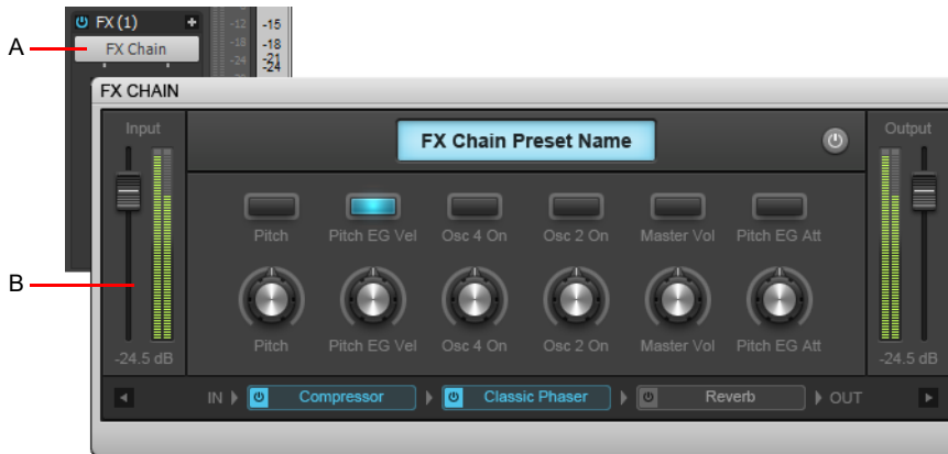
A. FX Chain container in FX Rack B. FX Chain property page
