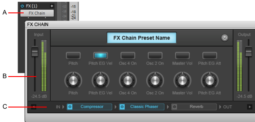
A. FX Chain container in FX Rack B. FX Chain property page C. Right-click to add a new plug-in
