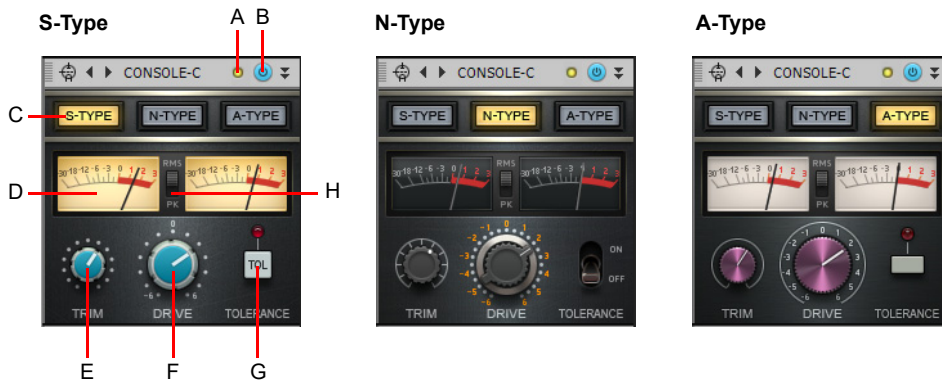
A. Clipping LED B. Console Emulator enable/disable C. Emulation mode D. Output VU meters (left and right channels) E. Trim (not available in bus module) F. Drive G. Tolerance H. RMS/Peak meter toggle
