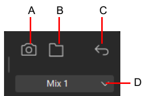
A. Save Scene B. Save As New Scene C. Recall Previous Scene D. Mix Recall menu
