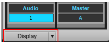
Figure 335. Use the Display menu to configure modules in the Track Inspector.
