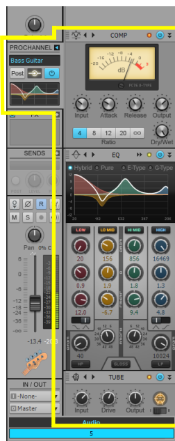
Figure 468. ProChannel provides compressor, equalizer, tube saturation, console emulation, tape emulation, and convolution reverb processing for each channel.
